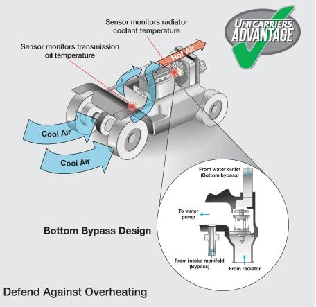
Our reliable cooling system includes an electronic engine protection and warning system that **monitors radiator fluid and transmission oil temperatures at all times.** This system also contains a field-proven bottom bypass design with thermostat to **prevent hot spots and prolong engine life.** And its large 10-blade fan and aluminum radiator produce effective cross-flow cooling.
